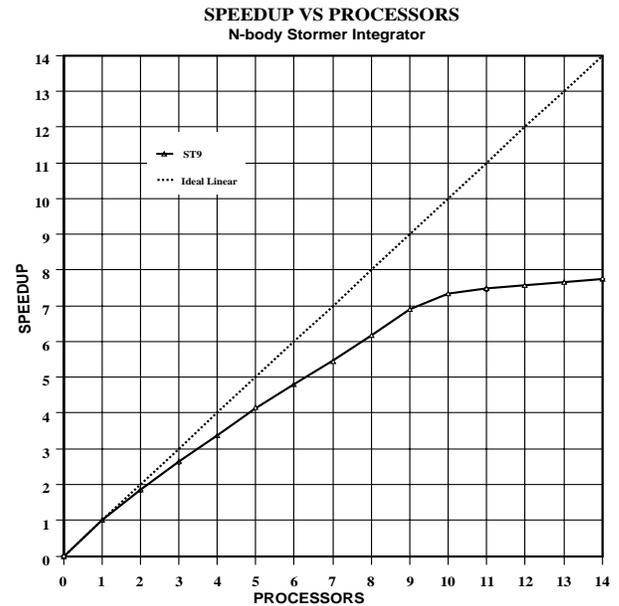
Figure 9: Speedup graph of Stormer integrations. Ample speedups are available to keep the 8-processor *Supercomputer Toolkit* busy, However, the incremental improvement of using more than 10 processors is relatively small.
