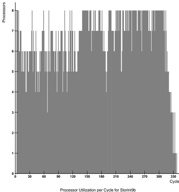
Figure 8: The result of scheduling the 9-body problem onto 8 *Supercomputer Toolkit* processors. Comparison with with the region-level parallelism profile (figure 6) illustrates how the scheduler spread the course-grain parallelism across the processors. A total of 340 cycles are required to complete the computation. On average, 6.5 of the 8 processors are utilized during each cycle.
